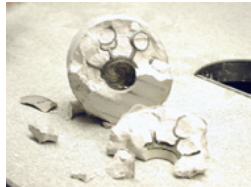
After devesting and cleaning . . .
