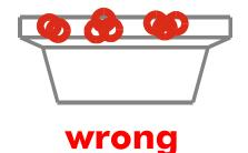
It is important to avoid sprueing to a center sprue base but to mount each sprue radially to the waxdisk. To avoid turbulences and insufficient flow the sprues should be fixed side by side without any overlap (see illustration above).
