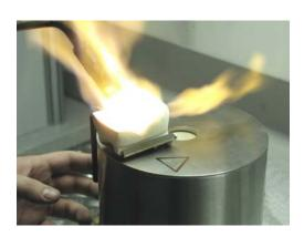
After reaching the liquidus point of the metal it may be poured into the mould by turning the crucible holder handle **13** in a smooth move to tip over the crucible **11**.
