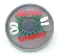
To prevent air bubbles it is important that the parts are fixed with the open side on top or at least parallel to the mould socket base.
