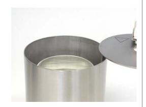
Unscrew the three mounting screws of the mould holder with the small key (part of delivery). Take the mould holder and the 3 cm high adapter-ring underneath out of the device.
