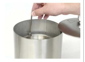
Place the mould holder without the adapter-ring in the device and fix it by hand with the three short screws at equal torque.
